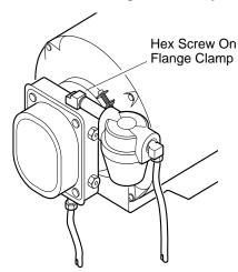
Figure 11 - Location of Screw on Flange Clamp
